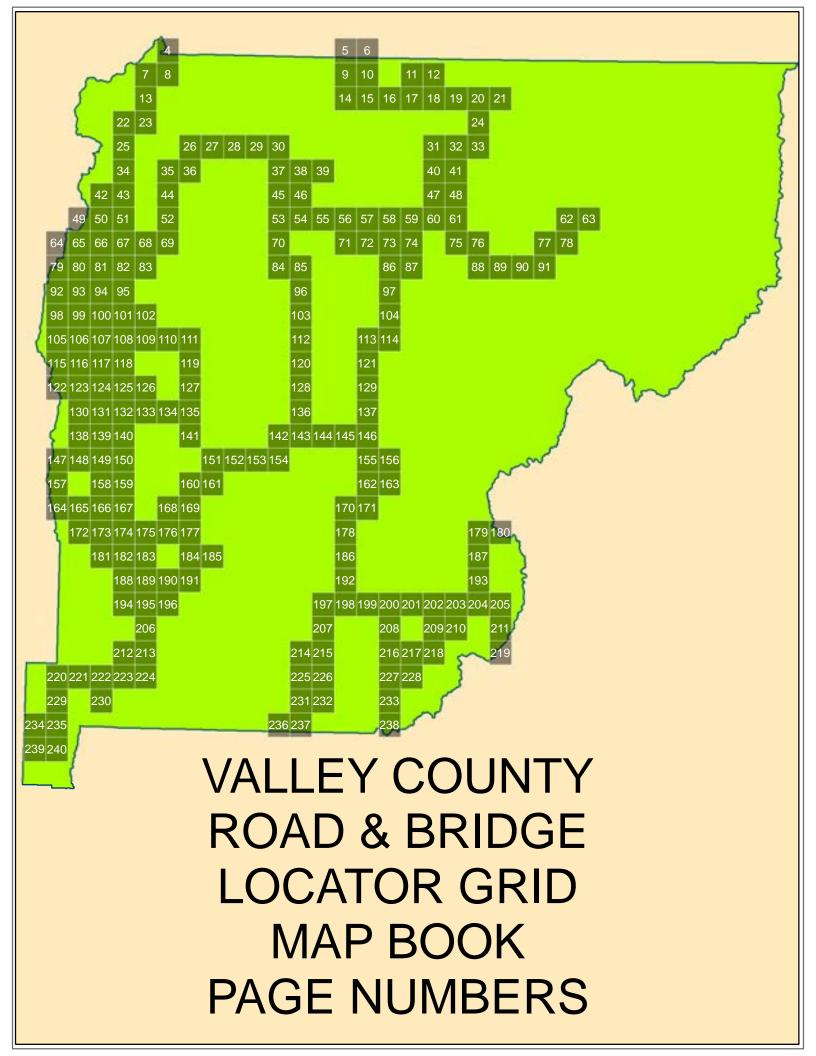
Coordinate System: NAD 1983 Idaho TM Projection: Transverse Mercator Datum: North American 1983 False Easting: 2,500,000.0000 False Northing: 1,200,000.0000 Central Meridian: -114.0000 Scale Factor: 0.9996 Latitude Of Origin: 42.0000 Units: Meter
