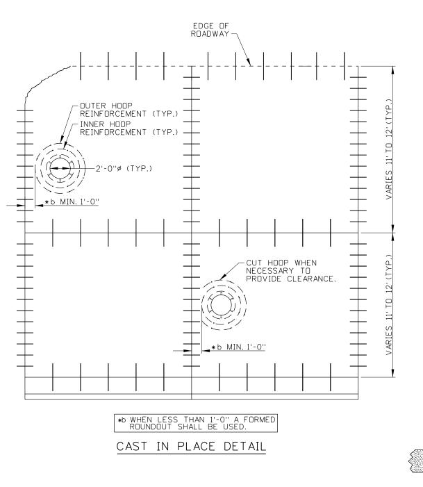
\*16 BARS. 6" LONG TO BE POUNDED INTO SUBGRADE AS CHAIRS & TIED. (MIN. OF (4) FOR INNER LOOP & (8) OUTER LOOP). INNER LOOP MAY REST DOWEL BAR (TIE BAR TO LONGITUDINAL JOINT) OR TIE BARS WHICH SHALL NOT INTERFERE IN THE ALIGNMENT.
