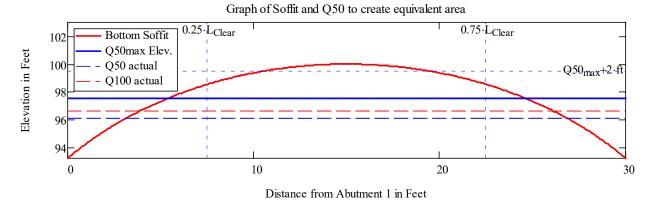
All multi-span beam type bridges should have a minimum 2' clearance above Q50 elevation at all points. In addition, the Q100 elevation shall be less than the lowest girder soffit elevation of the structure.
