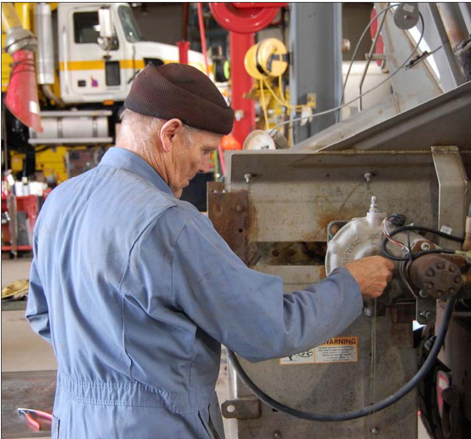
Shop Mechanic Darwin Palmer changes out the sander-chain motor on a plow truck.
