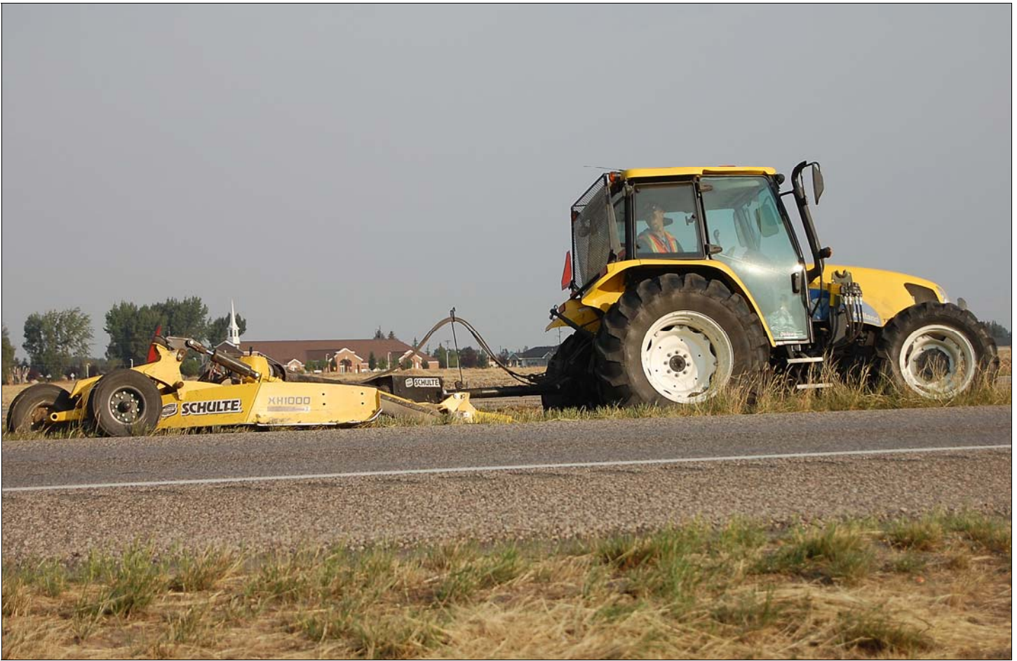
Transportation Technician Reagan Hansen mows the U.S. 20 roadside south of Rigby. Mowing reduces snowdrifts in the winter.
