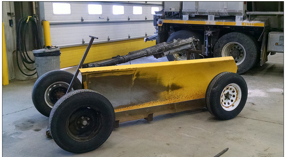
This dolly eliminates the need for a loader and its operators to install snowplow blades.
