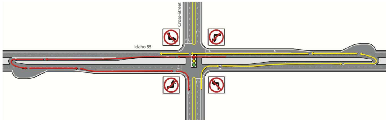
Figure A-10. Option 2 – median U-turn (MUT) intersection
