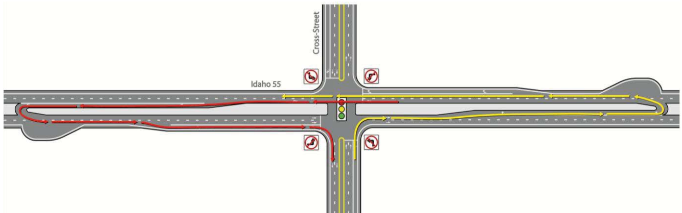
Figure 16. Preferred intersection alternative – median U-turn (MUT) intersection
