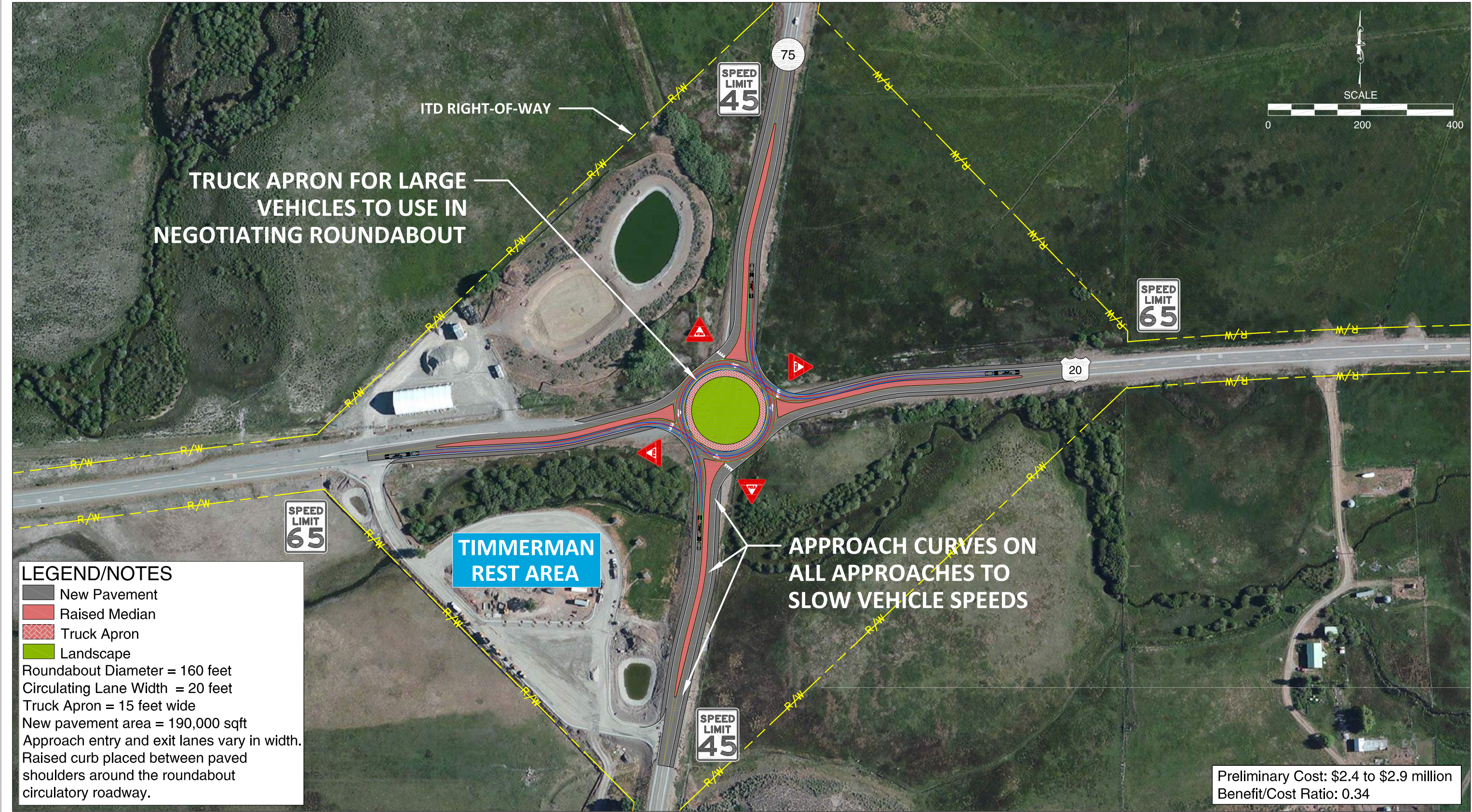
WB-67 Truck Turns from US-20 onto SH-75 Single-Lane Roundabout with Approach Curvature Blaine County, Idaho
