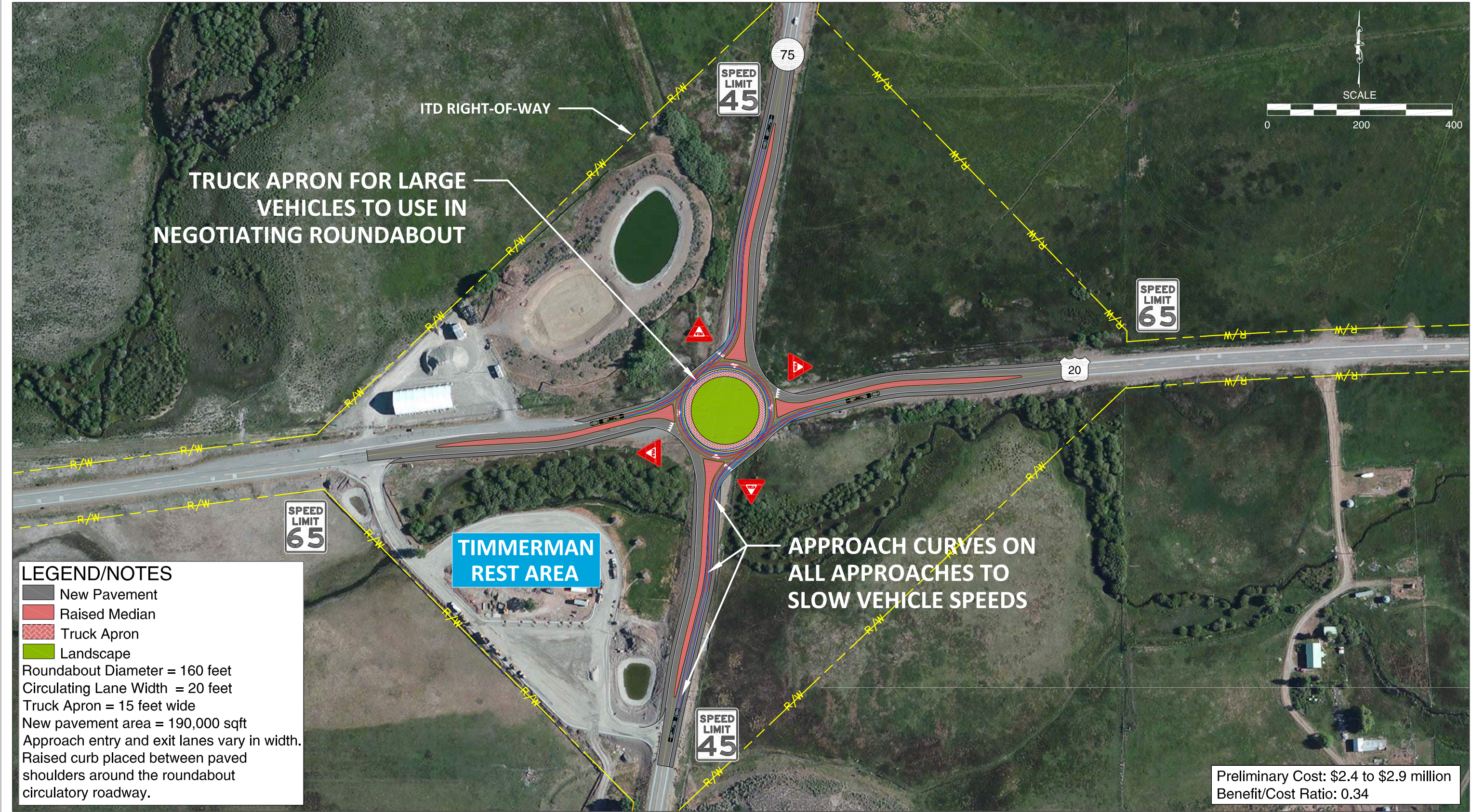
WB-67 Truck Turns from SH-75 onto US-20 Single-Lane Roundabout with Approach Curvature Blaine County, Idaho
