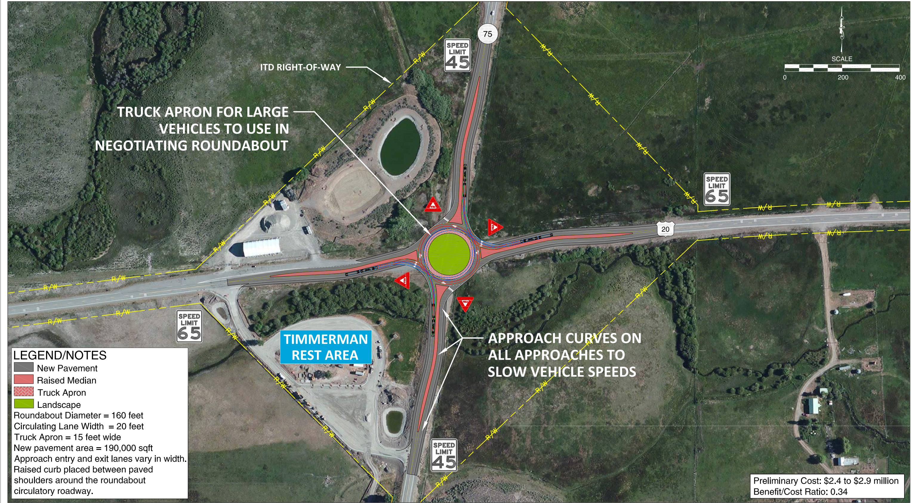
WB-109 Truck Turns from US-20 onto SH-75 Single-Lane Roundabout with Approach Curvature Blaine County, Idaho
