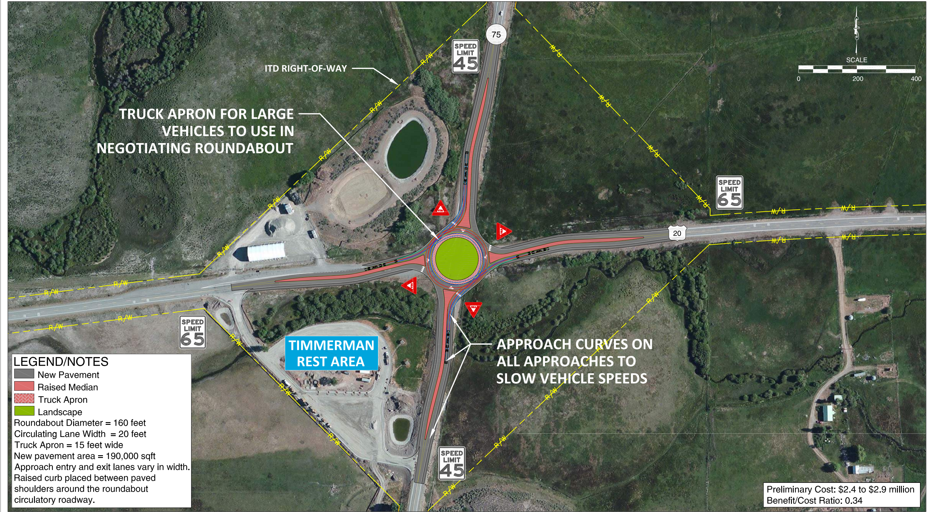
WB-109 Truck Turns from SH-75 onto US-20 Single-Lane Roundabout with Approach Curvature Blaine County, Idaho
