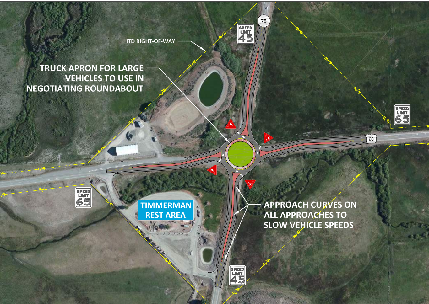
Exhibit 18. Single-Lane Roundabout with Approach Curvature Concept & Assessment
