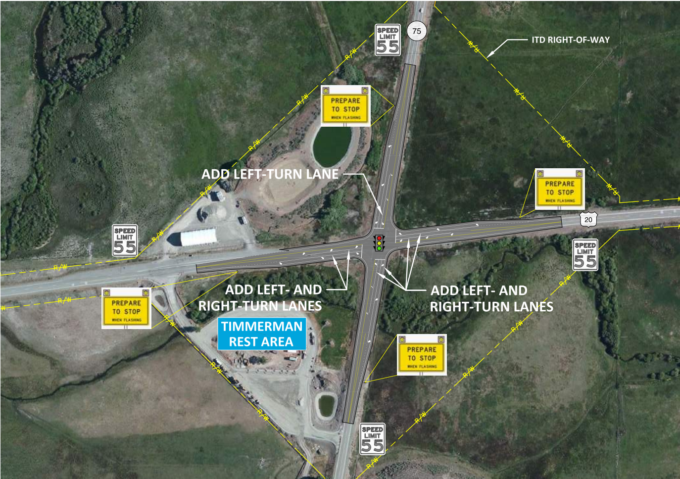
Exhibit 16. Traffic Signal with Addition of Turn Lanes Concept & Assessment
