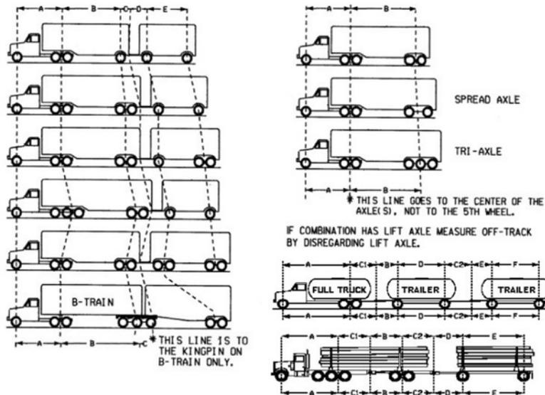
Figure 15: An example of a 129,000-pound truck configuration with the corresponding offtracking value.
