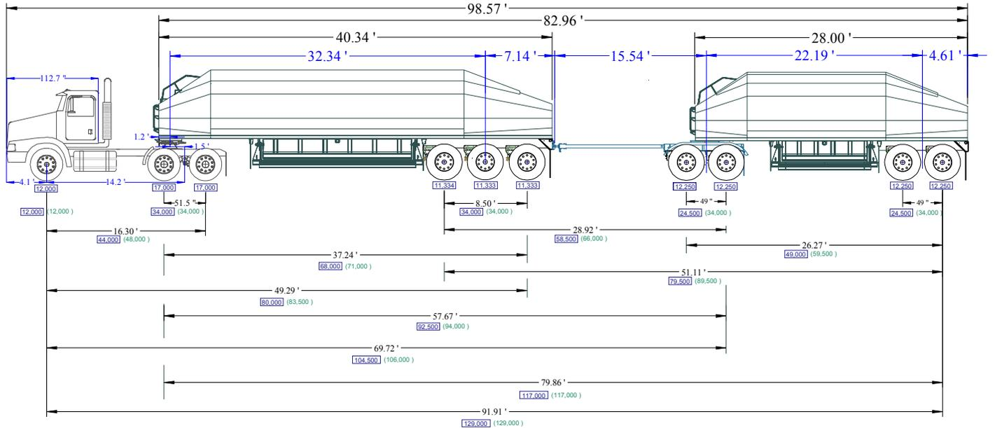
Figure 6: Transsystems 129,000K Truck Configuration Offtracking = 5.81 feet
