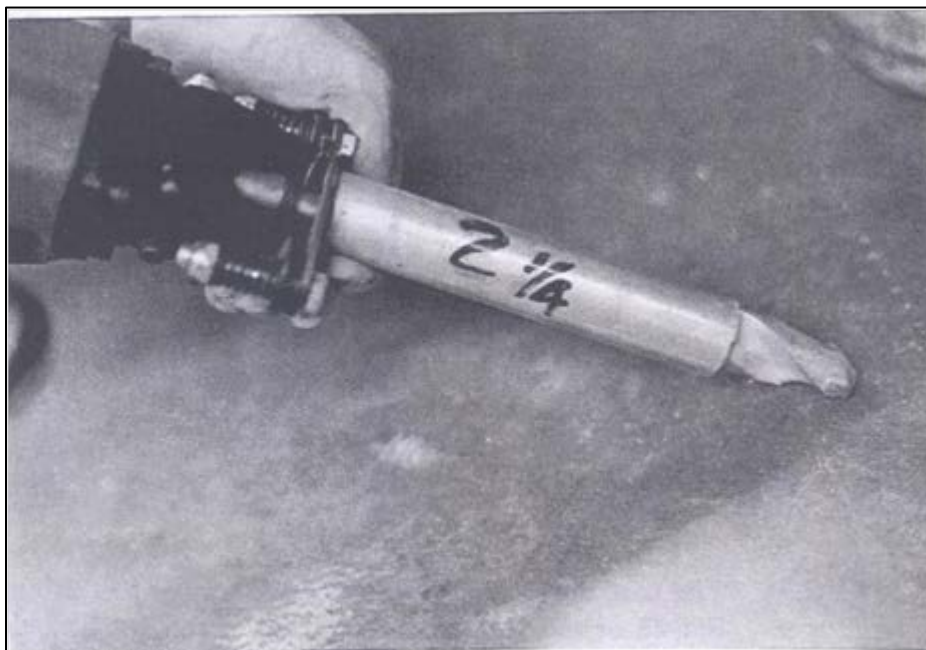
Illustration F: Rotary hammer with depth sleeve in place. Ready to drill sample. Clean drill bit, depth sleeve, and sampling spoon between sample depths with 2- Propanol.
