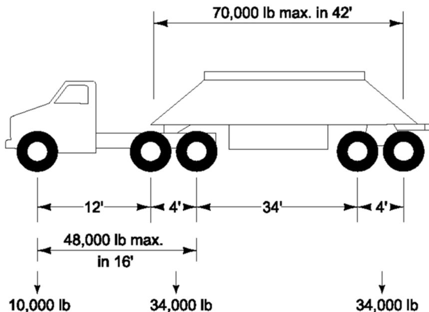
In 16 ft., three axles can only have 48,000 lbs. and two tandem axles can only carry 68,000 lbs. under [49-1001\(1\)](#). Therefore, the truck is okay. In 42 ft., four axles can have 70,000 lbs. but cannot exceed legal axle weights; in this case 34,000 lbs. on tandems. [49-1001\(2\) and \(9\)](#) will allow greater weights on the tandem axles. The front axle could carry 3,500 lbs. additional load and be legal. However, the front axle cannot exceed 600 lbs. per inch of tire width.
