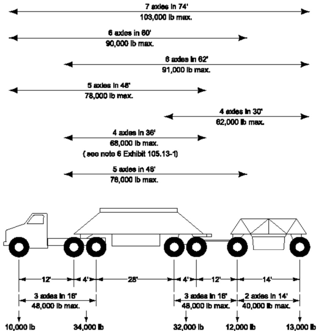
The overall spacing is usually not a problem, unless a short wheel base tractor is used. Also the critical areas are the internal bridge measurements for axles 2-5 and 4-7.
