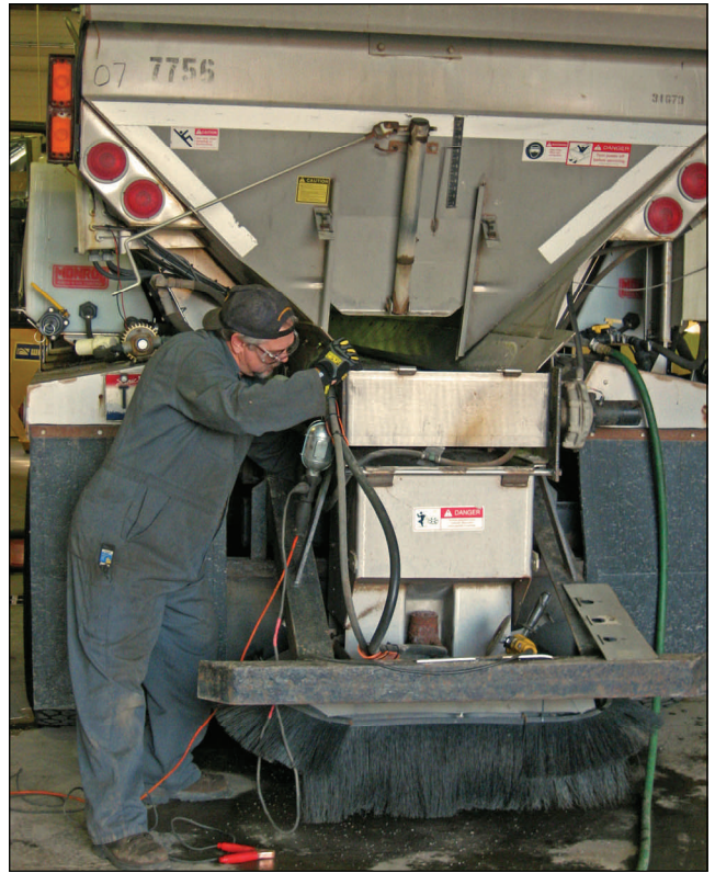
District 4 mechanic Ken Hall works out some of the kinks in a spreader in the Shoshone shop. Maintenance of the winter plows now begins following the rushed change-over season of the last month.
