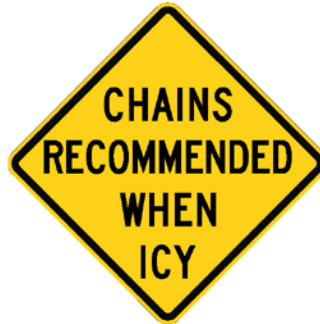
Figure 2C-4 Chains Recommended Sign
