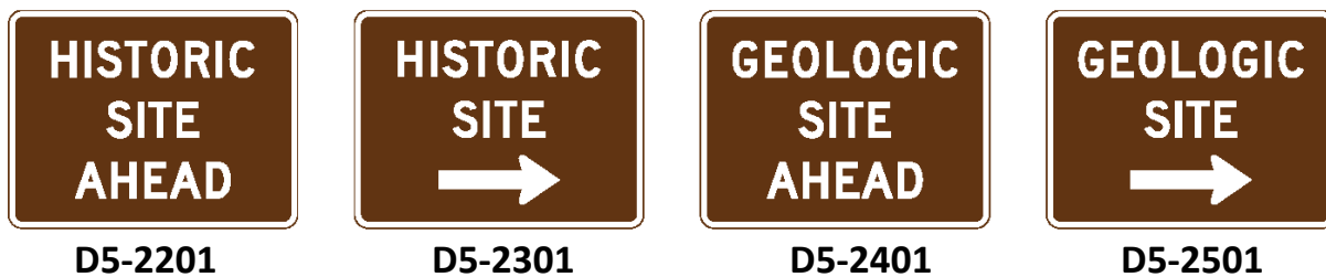
Figure 2M-3 Historic and Geologic Site Signs
