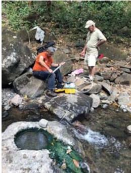
Left: Blackrock team obtaining water sample from thermal spring to test for helium. A peristaltic pump is used to extract water from a thermal spring to fill copper tubes with water to test for helium.
