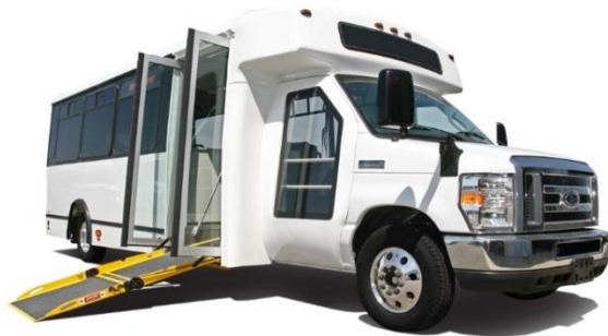
Low floor bus with ramp (Credit: Champion Bus)
