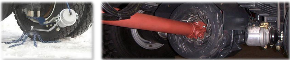
Auto chain system and driveline retarder system (Credit: left: ONSPOT; right: Telma)
