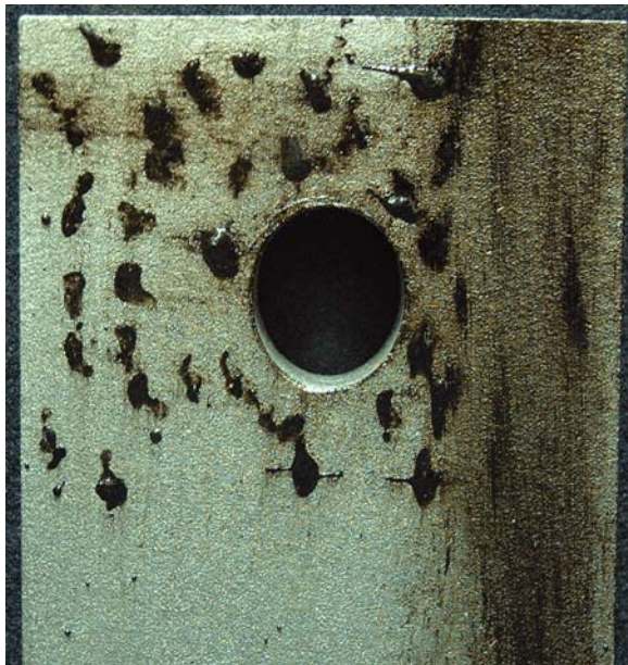
Figure 10. Effects of using wire brush in attempt to clean faying surface contaminated with chip seal oil.
