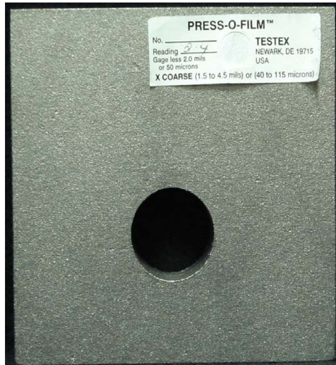
3Figure 3. Compression slip test specimen, blast cleaned surface.
