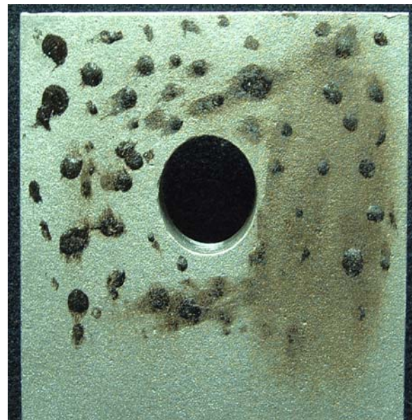
Figure 11. Effects of using 100 percent Acetone in attempt to clean faying surface contaminated with chip seal oil.
