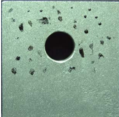
7Figure 7. Specimen Contaminated with Chip Seal Oil (CRS-2P).
