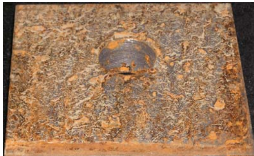
6Figure 6. Clayey-Mud and Magnesium Chloride.
