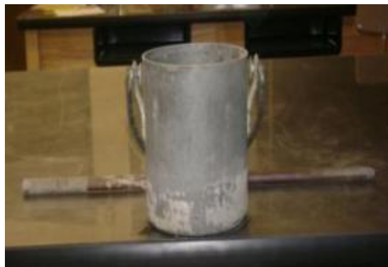
Figure 61. Equipment Used for the Aggregate Loose Unit Weight Experiment
