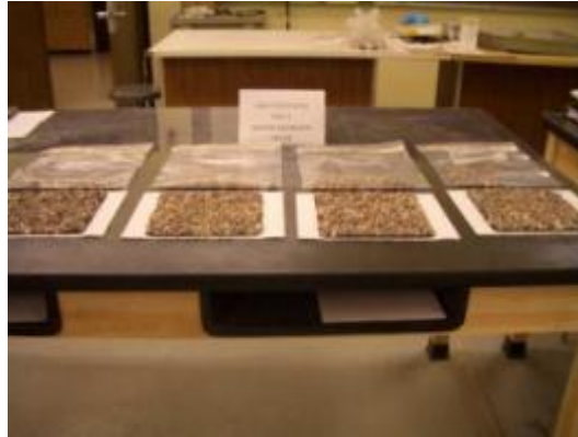
Figure 81. Vialit Test Plates After Tests Were Performed for Washed ITD District 5 Aggregate and CRS-2R Binder
