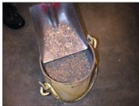
Figure 16. Loose Unit Weight Bucket and the Scoop
