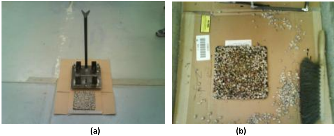
Figure 22. Vialit Test with Aggregate and Binder Sample, (a) Before and (b) After the Impact of the Ball
