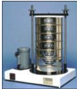
Figure 10. Sieve Shaker with Sieves
