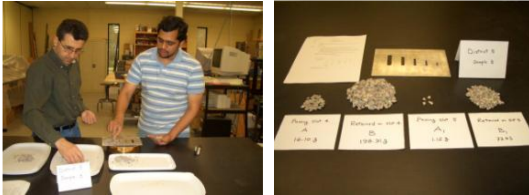
Figure 15. Conducting the Flakiness Index Test on ITD District 5 Aggregate
