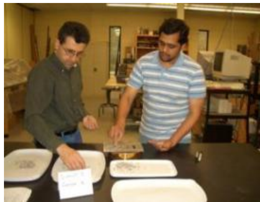
Figure 59. Flakiness Index Test Being Performed by Placing the Aggregate in the Slotted Plate
