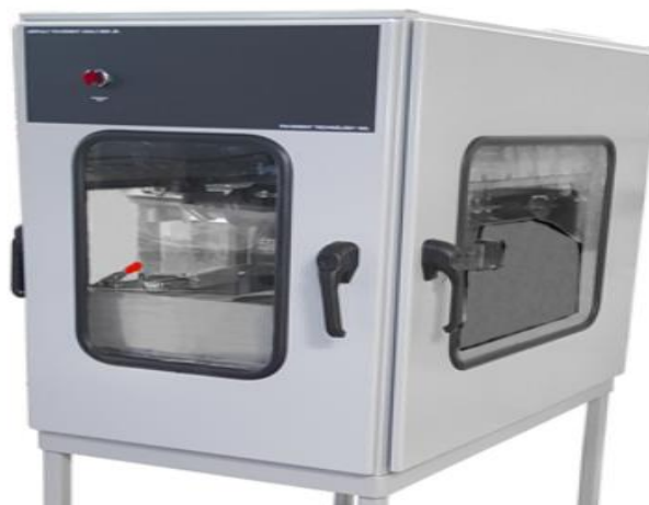
Figure 20. APA Jr. for Hamburg wheel tracking test
