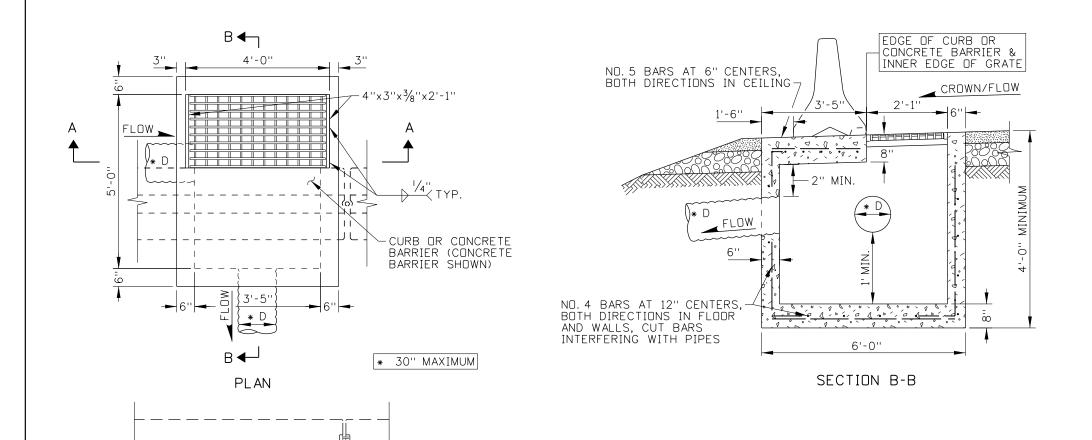
CURB OR CONCRETE BARRIER (CONCRETE
