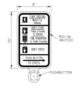
PEDESTRIAN PUSHBUTTON ASSEMBLY DETAIL SEE NOTE NO. 10
